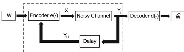
**Fig. 2** Diagram of a noisy channel. The capacity of the noisy channel without feedback is a function of  $I(X^n; Y^n)$ . With feedback, the capacity of the noisy channel changes. The capacity of the whole channel (inside the dotted line), which includes both the noisy channel and the feedback, is always a function of  $I(W; Y^n) = I(X^n \rightarrow Y^n)$
