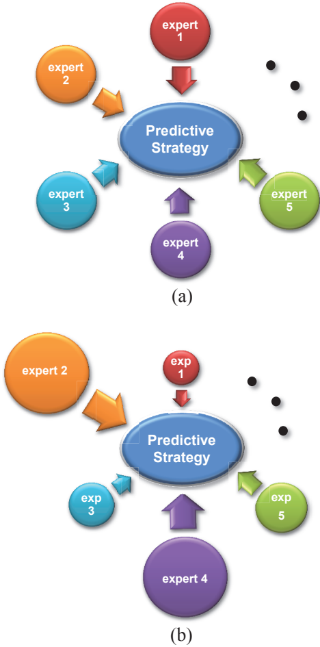
Fig. 3. Sequential prediction with expert advice: (a) Our own predictive strategy that is designed based on experts' advice. Initially, experts' advice is combined with equal weights. (b) Optimal predictive strategy. For each round we strategize how to combine these advice for experts with uneven weights so that the cumulative loss is getting close to that of the best expert in the class.
