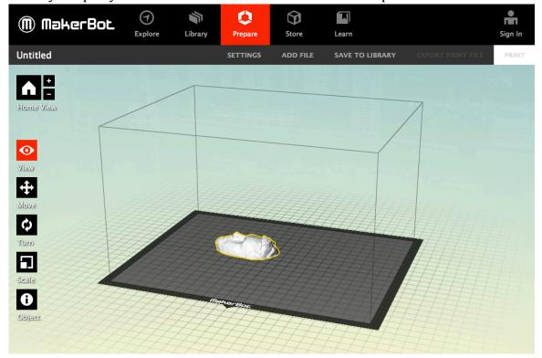
After opening, use the toolbar on the left to navigate. Click Scale and make sure the Uniform Scale button is checked. Next in scale, set the X dimension to 220 mm. The Y and Z should adjust accordingly.
