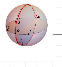
To find out how many zeros minus poles of a rational function in the right hemisphere are there, we can just count how many times the contour obtained by mapping the imaginary axis (run S->N) surrounds the origin clockwise.
