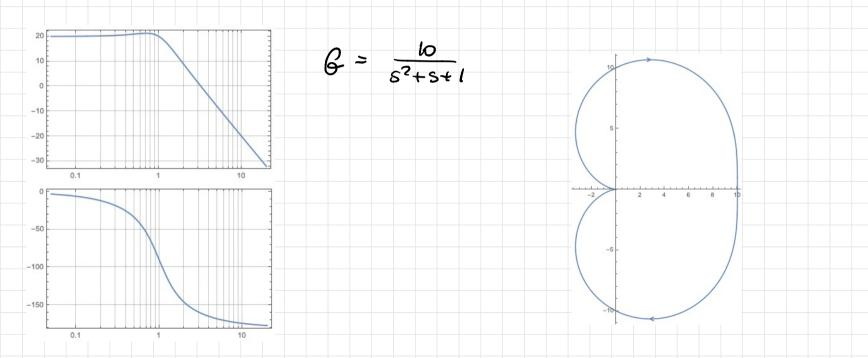
Particular usage of Nyquist plots: determine the number of RHP poles of the closed loop transfer function
