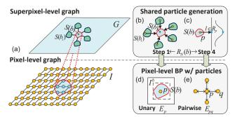
Figure 3. Two-layer graph structure used in SPM-BP: (b)(c) A superpixel-level graph generates new particle proposals  $\mathcal{R}_N(b)$  to be tested on the pixel-level graph (see **Step 1** and **Step 4** of Sec. 3.3). (d) For the reference superpixel S(b), the EAF is applied to obtain the data cost  $E_p$  for  $p \in S(b)$ . (e) The message passing algorithm proceeds in the inner loop of S(b) using (5), while outgoing messages on the boundary of S(b) are fixed.
