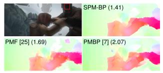
Figure 5. Visual and EPE comparison of the optical flow by PM-F [25], PMBP [7]. Note the errors in PMF's flow map.
