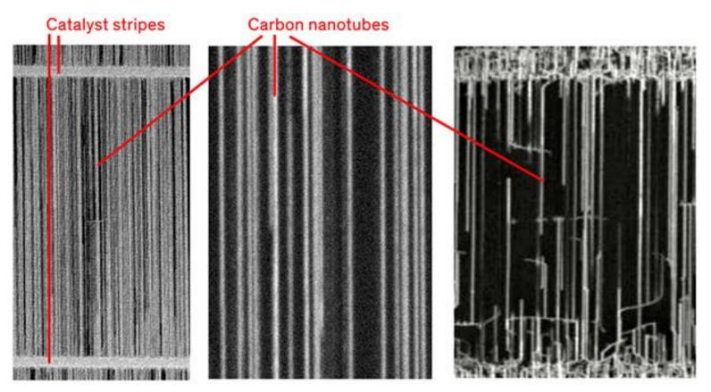
Carbon nanotubes can be grown in parallel lines, but imperfections do occur.
