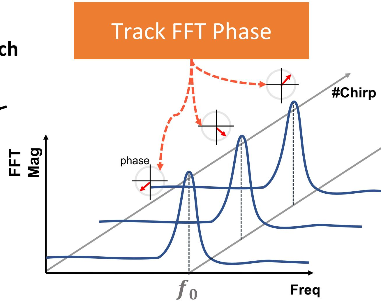
FMCW radar can also measure Vibration,
