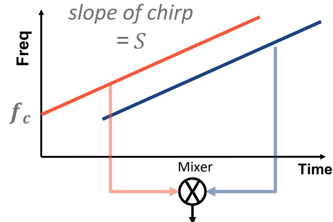
$$\begin{aligned}x(t) &= e^{j2\pi(S\tau(t)t + f_c\tau(t))} \\&= e^{j(2\pi f(t)t + \phi(t))}\end{aligned}$$
