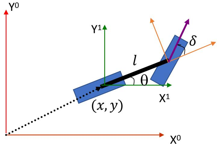
Plant state: real wheel pose) =  $\mathbf{x}_B: \mathbb{R}^3 = \begin{bmatrix} x_B \\ y_B \\ \theta_B \end{bmatrix}$
