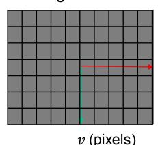
Pixels may be rectangular Let  $m_x$  and  $m_y$  be the pixel densities (pixels/mm) in x and y directions
