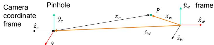
Given the extrinsic parameters  $(R, c_w)$  of the camera, the camera-centric location of the point P in the world coordinate is
