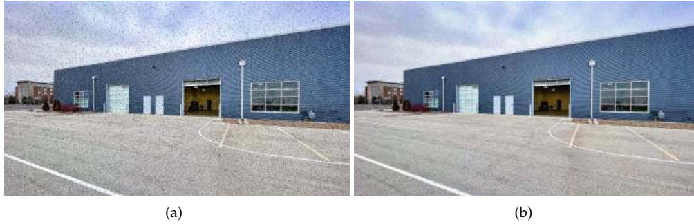
Figure 2: (a) Salt and Pepper Noise (b) Gaussian (White) Noise
