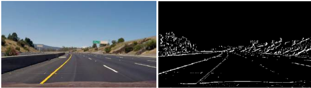
Figure 6: Image gradient. Left: Original image. Right: Gradient image.
