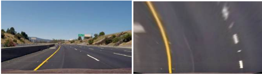
Figure 8: Perspective transformation. Left : Original image. Right : Bird's eye view image.
