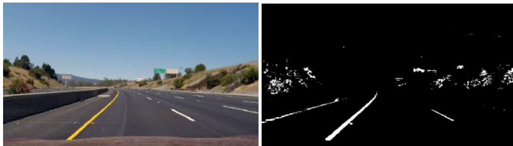
Figure 7: Color threshold. Left : Original image. Right : Color threshold image.
