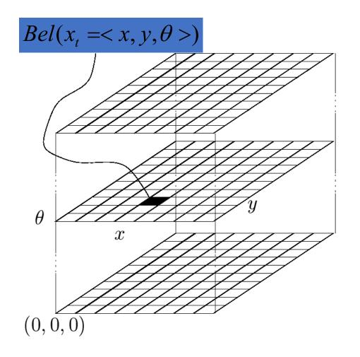
Fixing an input u<sub>t</sub> we can compute the new belief
