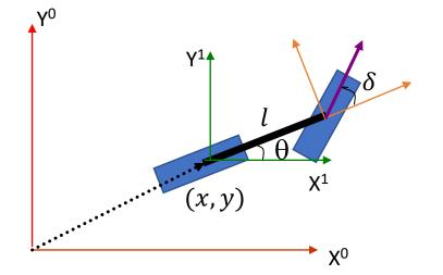
Car length = lCar (real wheel) pose =  $\begin{bmatrix} x \\ y \\ \theta \end{bmatrix}$ Car speed = vCar (front wheel) steering angle =  $\delta$
