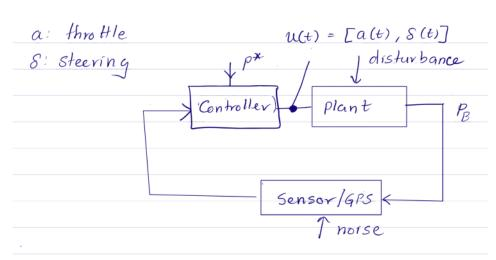
Now you can apply PID or state-feedback control after linearization
