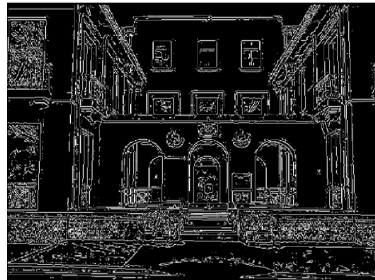
low threshold (weak edges)
