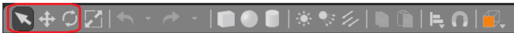
Figure 3: The buttons in the red box from left to right are selection mode, translation mode and rotation mode.
