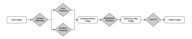
Figure 4: Lane detection module overview.
