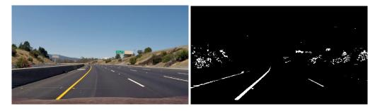
Figure 6: Color threshold. Left: Original image. Right: Color threshold image.
