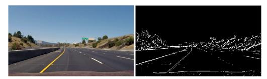
Figure 5: Image gradient. Left: Original image. Right: Gradient image.
