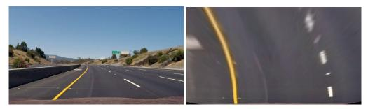
Figure 7: Perspective transformation. Left: Original image. Right: Bird's eye view image.
