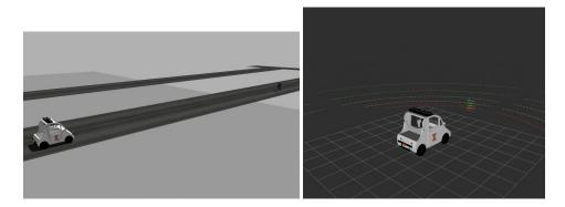
Figure 1: Vehicle and pedestrian on a single lane. *Left:* Initial positions of the two are at  $x_{10}$  and  $x_{20}$ , respectively. *Right:* Vehicle undergoes constant deceleration  $a_b$  once the pedestrian is detected by the vehicle.
