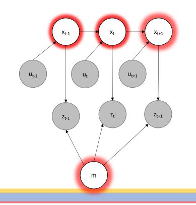
Shaded known: control inputs (u), measurements(z). White nodes to be determined (x,m)
