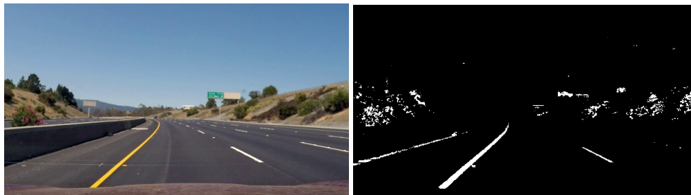
Figure 5: Color threshold. Left: Original image. Right: Color threshold image.
