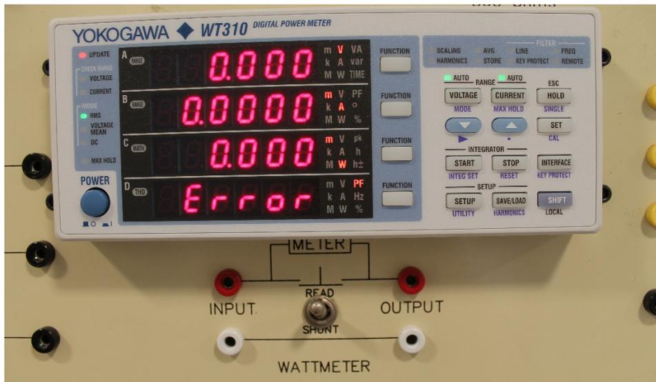
Figure 6. Front panel view of Yokogawa model WT310 meter, mount, and connections.
