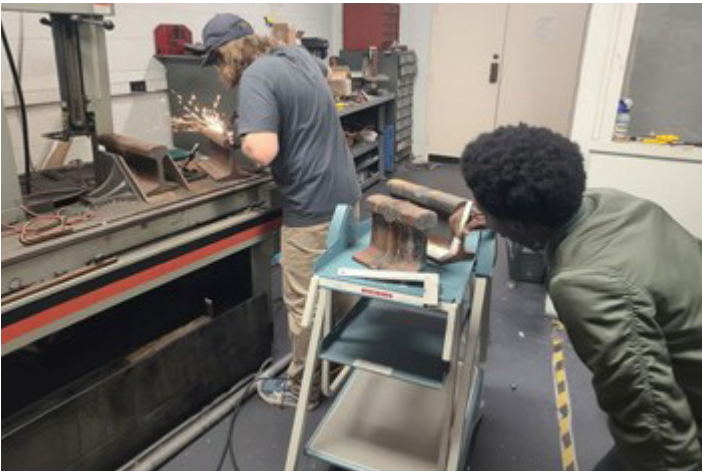
Grinding of railhead of thermite welded samples.
