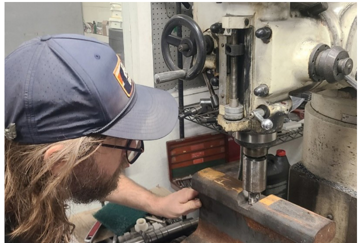
Milling of a rail section insert before GMAW welding.
