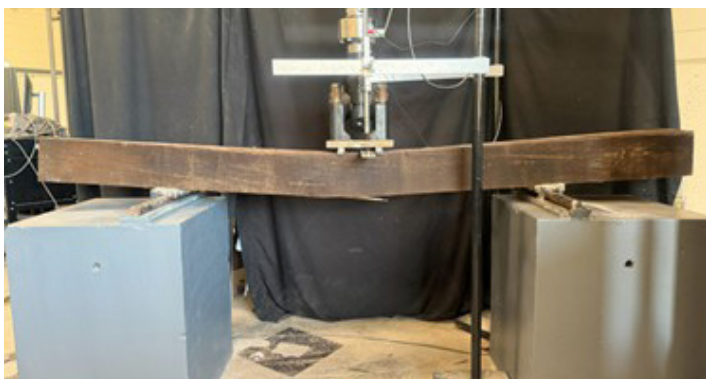
Wood Tie Deflected Failure Point
