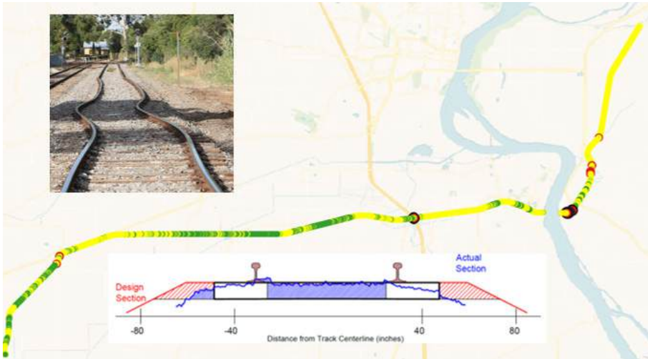
Example visualization of the IBRM's output in a track segment color-coded based on the associated risk at a tie-by-tie level.
