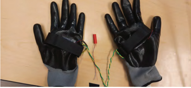
Fig. 5: Vibrotactile feedback gloves worn by the teleoperator with vibrotactors in the center of the palm secured by a strap to ensure sensation transmission to the operator.
