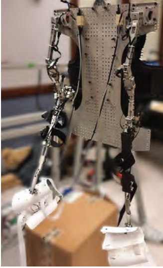
Fig. 3: Human motion capture system with back-plate, vest mounting, and two arms attached to the human with the white forearm braces allowing hands-free operator measurement.
