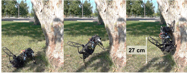
Fig. 10. Pinto performing a tree jump, raising its center of mass about a body length above the ground at the time of contact.
