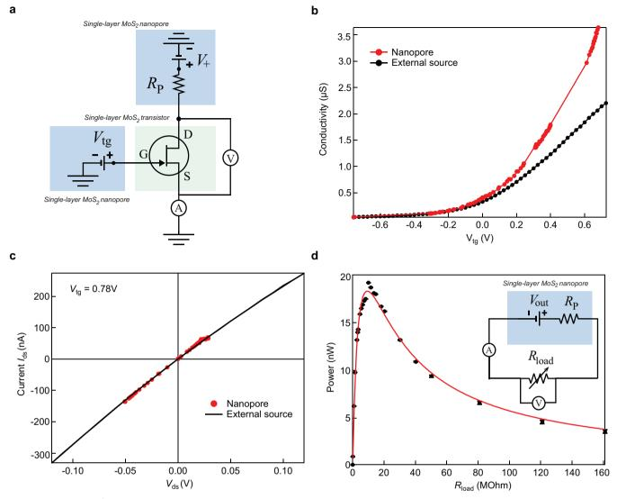
**Extended Data Figure 8** | **Characterization of a single-layer MoS<sub>2</sub> transistor with nanopores and SMU. a**, Electrical measurements with two nanopores ( $V_+$ , nanopore output voltage;  $V_{ds}$ , drain–source voltage;  $V_{tg}$ , top gate voltage). The voltage drop across the transistor channel is monitored with the voltmeter (V); current is measured with current amplifier (A). b, Comparison of nanopore measurements with
