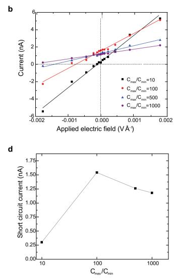
Extended Data Figure 4 | Molecular-dynamics simulations of power generation for various ratios of concentration gradients. a, A typical simulation box. b, Current as a function of the applied electric field for a single-layer  $MoS_2$ , at different concentration ratios. c,  $K^+$  and  $Cl^-$
