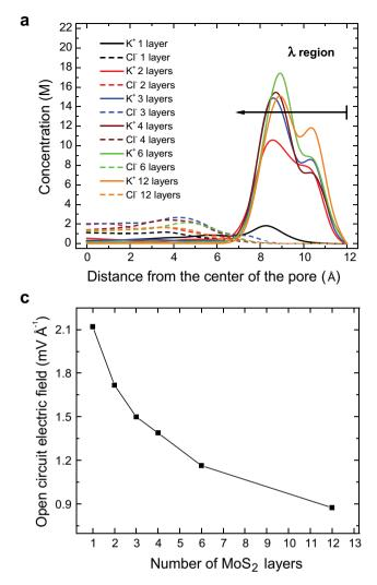
Extended Data Figure 7 | Simulated power generation as a function of membrane thickness. a,  $K^+$  and  $Cl^-$  concentrations as a function of the radial distance from the centre of the pore for single-layer and multilayer membranes. The  $\lambda$  region, near the charged wall of the pore, is representative of the electrical double layer. **b**, The mobility of each
