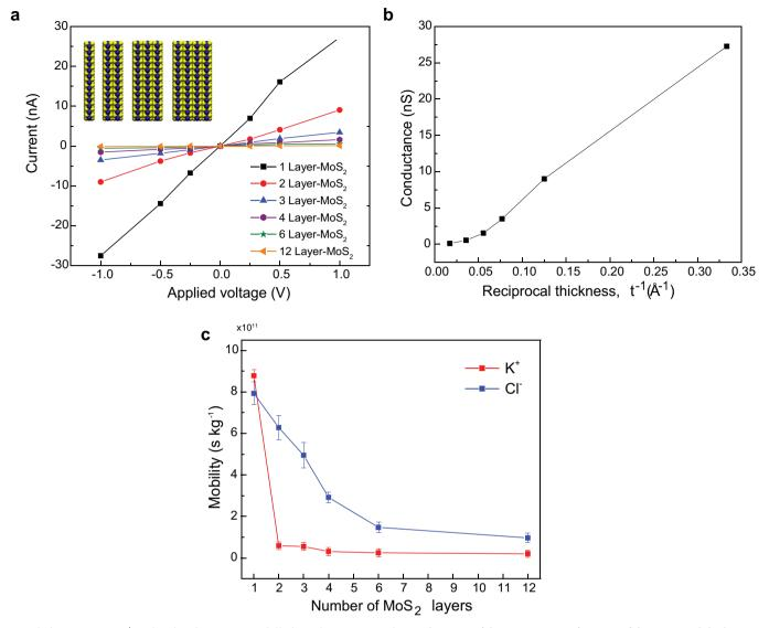
**Extended Data Figure 6** | Molecular-dynamics-modelled conductance as a function of membrane thickness. a, I-V curves for six membranes with a different number of  $MoS_2$  layers, across a symmetrical 1 M KCl solution. The inset illustrates simulated multilayer membranes.
