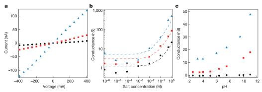
Figure 2 | Electrical conductance and chemical reactivity of the  $MoS_2$ nanopore. a, Current–voltage response of  $MoS_2$  nanopores with different pore sizes (black, 2 nm; red, 6 nm; blue, 25 nm) in 1 M KCl at pH 5. b, Conductance as a function of salt concentration at pH 5. By fitting the
