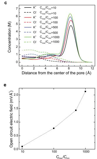
concentrations as a function of the radial distance from the centre of the pore, for different concentration ratios. **d**, Short-circuit current as a function of the concentration ratio. **e**, Open-circuit electric field as a function of the concentration ratio.
