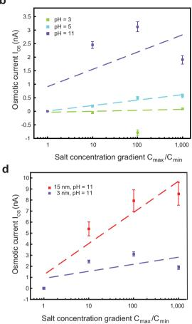
Extended Data Figure 2 | Dependence of osmotic power generation on pH and pore size. a, b, Osmotic potential (a) and osmotic current (b) generated using a 3-nm pore under different pH conditions (pH 3, 5 or 11) and in different concentration gradients. Power generation (both osmotic potential and osmotic current) at pH 3 is very low and sometimes
