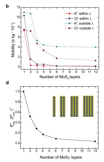
ion type within and outside the  $\lambda$  region for different layers of membranes. c, The open-circuit electric field across the membrane for different numbers of MoS<sub>2</sub> layers. d, Ratio of the maximum power (*P*) generated by multilayer membranes to the maximum power generated by a single-layer membrane, for different numbers of layers.
