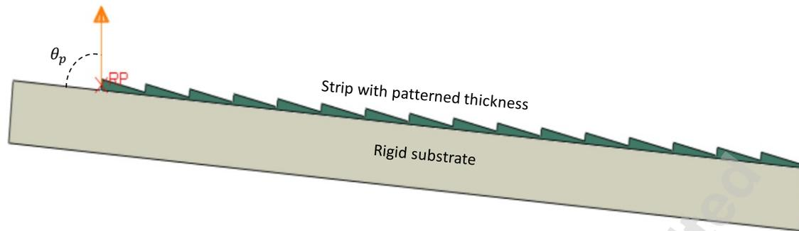
Fig. 5: Model setup for the finite element analysis. A homogenous thin film with saw tooth thickness profile is peeled from a rigid substrate. The peeling angle is  $\theta_p$ .
