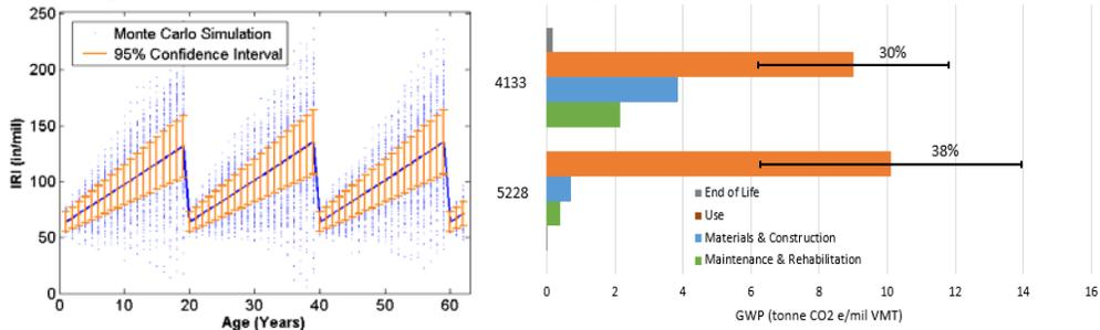
**Figure 2. (a) IRI Progression with uncertainty band and (b) Resulting use stage output range**
