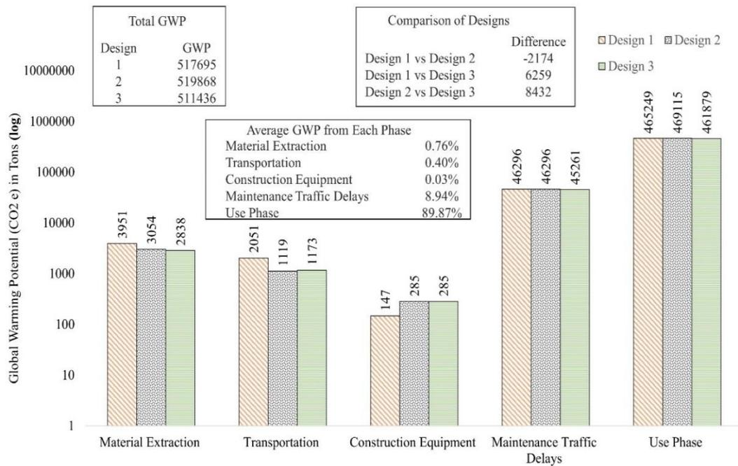
Figure 3. GWP of Three Pavement Designs (Deterministic Approach)
