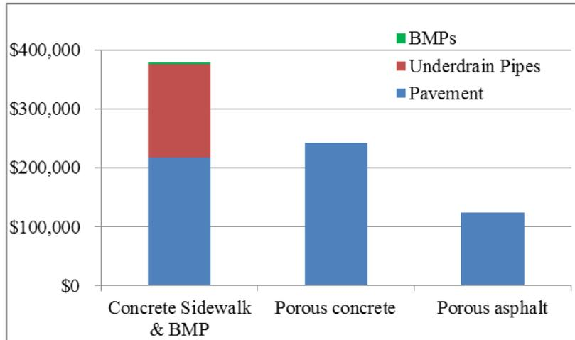
Figure 3 Initial construction cost (\$/mile) of three sidewalk pavements
