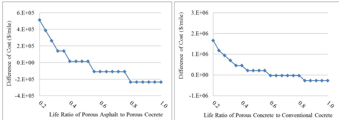
Figure 4 Breakeven points of pavement life ratios between (a) porous asphalt and porous concrete and (b) porous concrete to conventional concrete for cost (\$/mile) (the life of porous concrete is assumed to be 25 years in 40-year analysis period)
