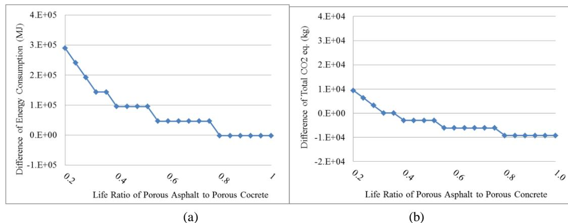
Figure 2 Breakeven points of pavement life ratios between porous asphalt and porous concrete (design 1 with slag cement) for (a) energy consumption and (b) CO<sub>2</sub> eq. emission (the life of porous concrete is assumed to be 25 years in 40-year analysis period)
