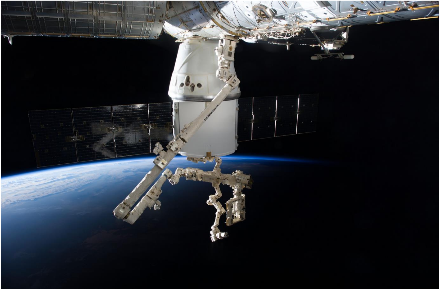
Figure 34: SSRMS on the ISS Reaching into the Dragon External Cargo Bay 84
