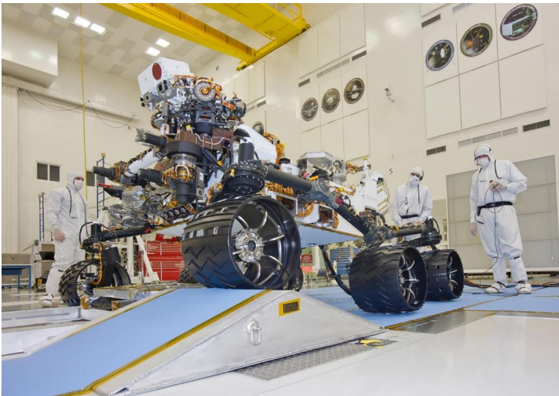
Figure 55: MSL Articulated Wheels and Traction Treads 126
