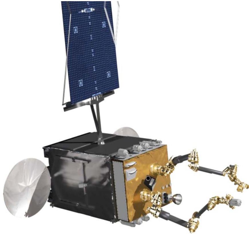
Figure 36: Illustration of the DARPA/SSL RSGS Vehicle
