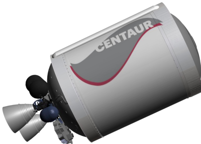
Figure 62: Advanced Centaur Upper Stage
