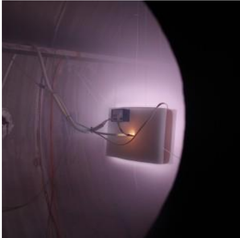
Figure 67: Vacuum Chamber Test of a 6U Cubesat-Scale MAC Demo System 150
