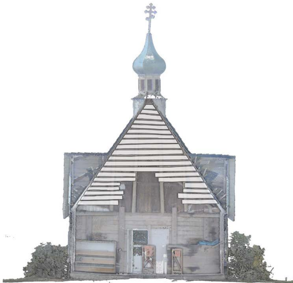
Figure 6. Laser scan data of the St. Nicholas Chapel in Kenai, AK. This section cut of the chapel highlights the unique roof construction and facilitated the planning efforts to maintain character defining features, such as the exposed rough sawn skip sheathing inside.
