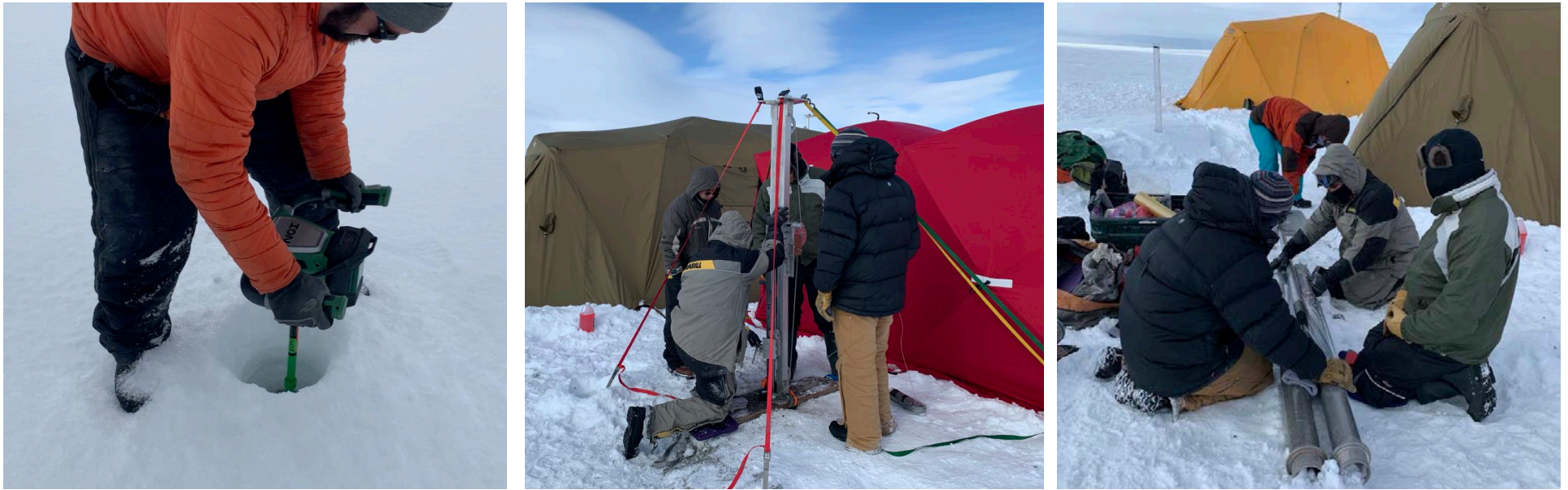
Figure 1. The lake coring process. A hole is drilled through the ice and a coring platform and a winching apparatus is placed above the hole. Sediment cores are extracted from the lakebed and extruded from the corer for later analysis in the laboratory. SKYDANCE AVIATION/SCOTT AMY
