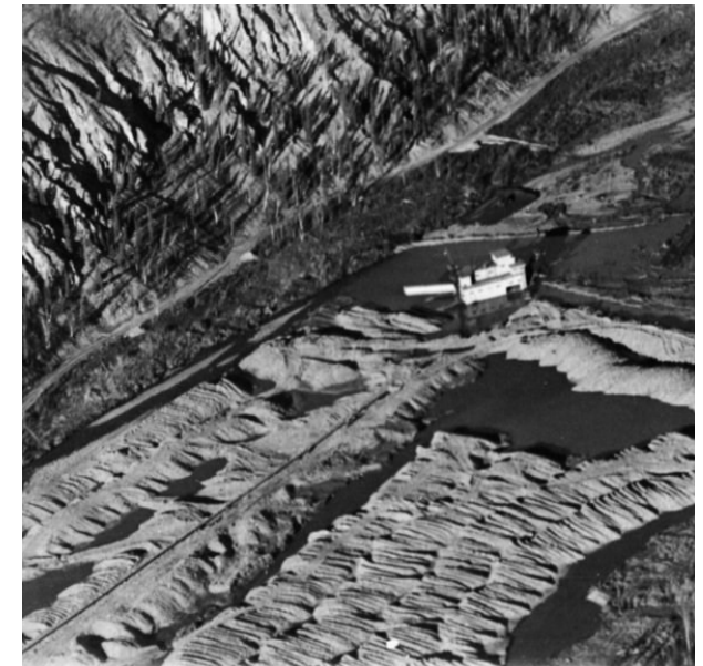
Figure 1. An aerial photo of Woodchopper Creek, Yukon-Charley Rivers National Preserve showing the effects of extensive dredge mining. NPS PHOTO
