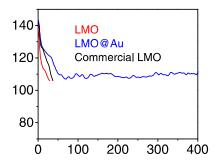
Figure 1: Discharge Capacity over 400 cycles for LMO, gold coated LMO( LMO@au) and commercial LMO at 1 C rate.
