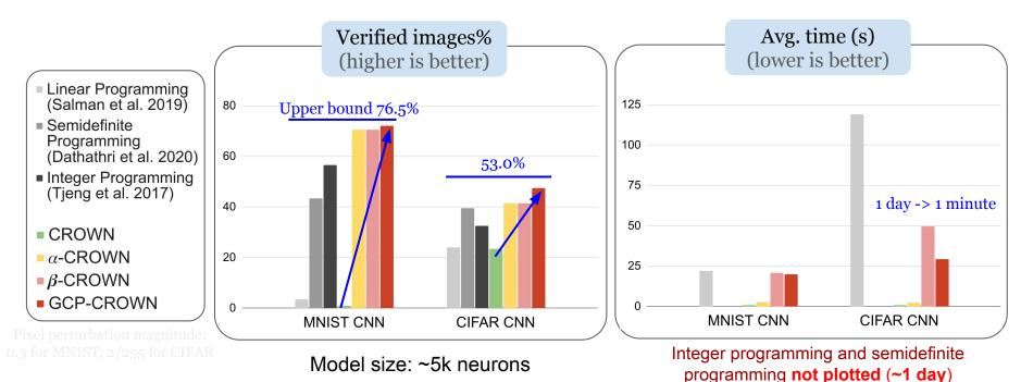
Key enablers: specialized bound propagation solver + GPU acceleration + BaB
