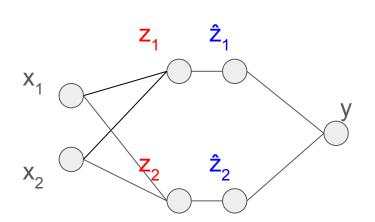
$$egin{aligned} y &\geq -rac{2}{3}z_2 - 2 \ z_1 &= x_1 - x_2 \ z_2 &= 2x_1 - x_2 \ y &\geq -rac{4}{3}x_1 + rac{2}{3}x_2 - 2 \end{aligned}$$
