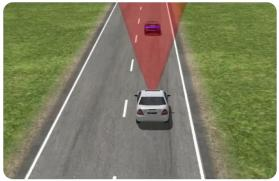
Verify no collision with uncertainties: speeds in [70, 85] mph and acceleration range of NPC
