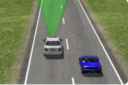
Verify no collision with **uncertainties** like speeds in [70, 85] mph and **bigger** acceleration range of NPC
