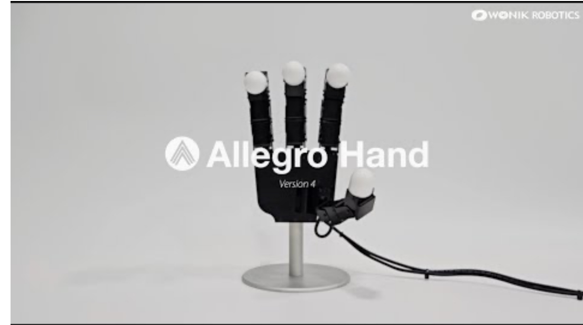
Allegro Hand. A fully actuated 4-fingered hand
