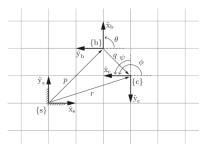
Let (R<sub>sc</sub>, r) denote the frame {c} with respect to {s} and (R<sub>sb</sub>, p) the frame {b} with respect to {s}. We can also represent {c} with respect to {b} as (R<sub>bc</sub>, q) (note that this is with respect to x<sub>b</sub>, y<sub>b</sub>!). Then we have
