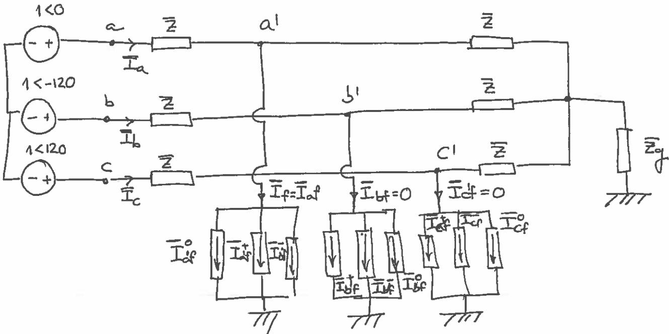
We can apply superposition and solve each sequence independently using per-phase equivalents
