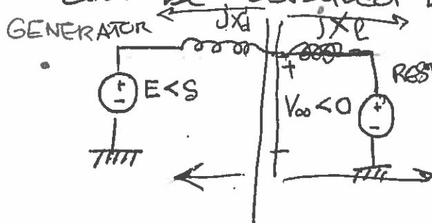
We derive the equation that governs the evaluation of  $s$  (the torque angle)
