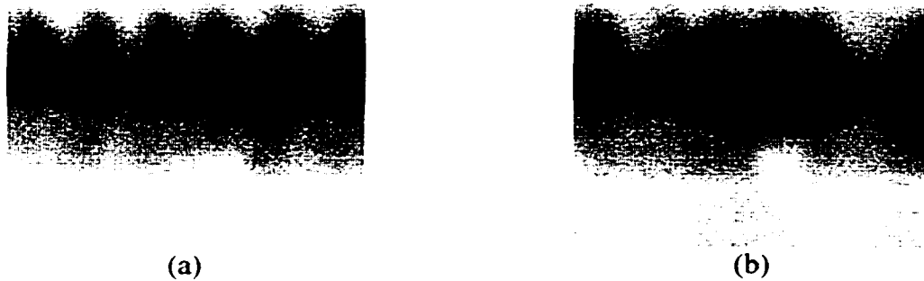
Figure 7.16: SSM images of flux instabilities in a 150\mu\text{m} wide, 110\text{nm} thick Nb strip with a 55\text{nm} surface step, such that the thin side of the strip is towards the top of the image. There is no external applied magnetic field, and transport currents are applied to the strip, triggering flux avalanches of flux bundles (dark regions) primarily into the thin part of the strip. The transport current was increased to (a) 99.1\text{ mA} , (b) 50.4\text{ mA} ( \approx 4 \times 10^5\text{ A/cm}^2 ). Image size = (254\mu\text{m})^2 .
