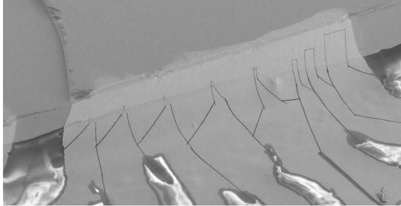
Figure 4.6: Initial attempt at fabricating Josephson Junctions using Focused Ion Beam Technology. Smallest junction on left is 500 \times 500 \text{ nm}^2 and each successive junction is doubled in size.
