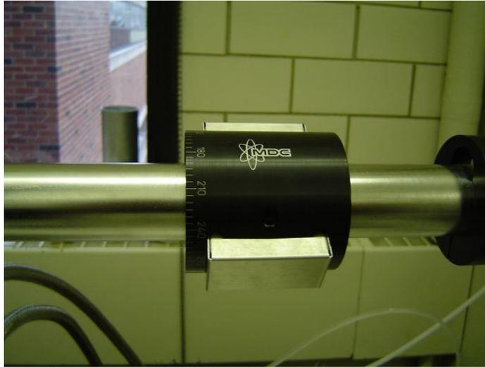
*Figure 4: Magnet used to adjust sample position*
