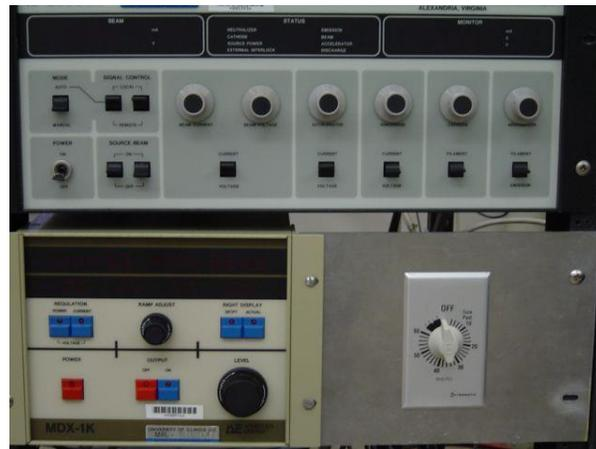
Figure 8: The ID 2500, MKS Flow Controller Model 2478, and water timer
