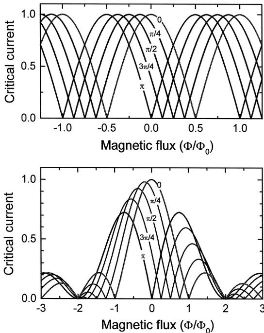
Fig. 7. Critical current modulation pattern expected for different intrinsic phase shifts for (a) SQUID and (b) single junction configurations.
