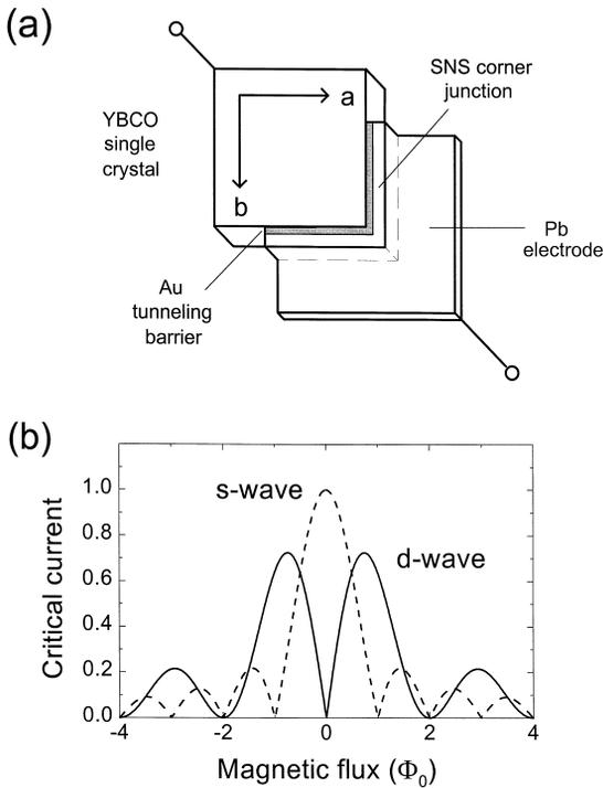
Fig. 2. (a) Modified interferometry experiment using a single corner Josephson junction straddling orthogonal faces of a superconductor sample. (b) Critical current modulation pattern vs. applied magnetic field for the corner junction with s and  $d_{x^2-y^2}$  order parameter symmetries.
