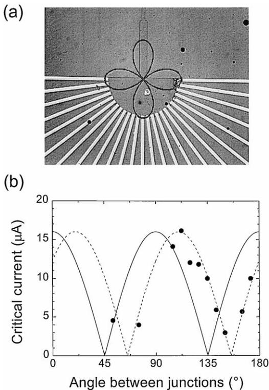
Fig. 4. (a) A series of Josephson junctions spaced every  $7.5^\circ$  on the edge of an oriented-YBCO thin film used to determine the angular anisotropy of the magnitude of the order parameter. Superimposed is the expected order parameter for  $d_{x^2-y^2}$  symmetry. (b) Critical current vs. angle for probes exhibiting a finite supercurrent. The solid line shows the expected variation for the  $d_{x^2-y^2}$  state; the dashed line is shifted by  $20^\circ$ .
