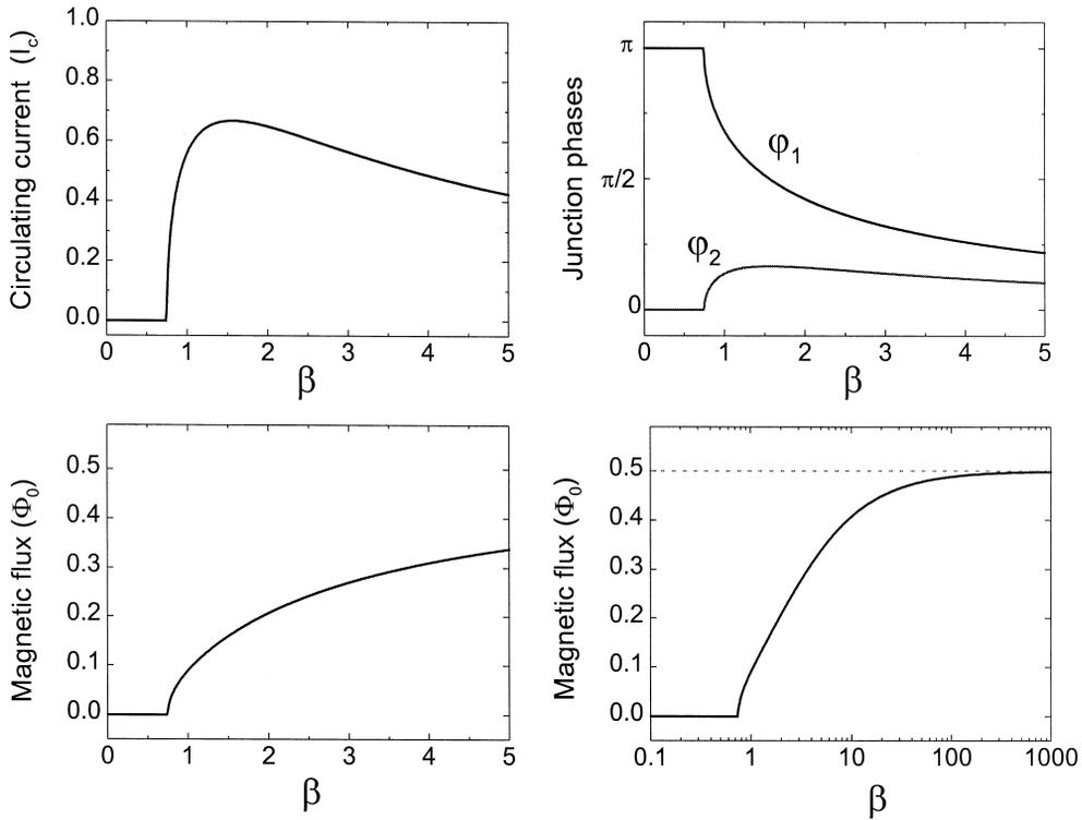
Fig. 5. Spontaneous circulating current, the resulting magnetic flux, and the phase drops across the junctions as a function of the inductance parameter  $\beta = 2\pi LI_c/\Phi_0$  for a critical current asymmetry such that  $I_{c1} = 2I_{c2}$ . For low  $\beta$ , the phase of one junction is  $\pi$  and no circulating current or flux is required to maintain the phase constraint.
