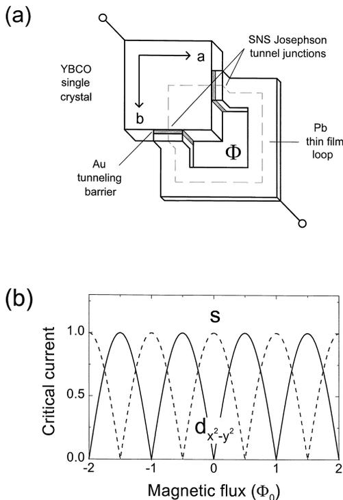
Fig. 1. (a) Configuration of the corner SQUID interferometry experiment in which a dc SQUID is formed by connecting Josephson tunnel junctions on orthogonal faces of superconductor sample with a conventional superconductor loop. (b) Periodic critical current vs. applied magnetic field for the corner SQUID with s and  $d_{x^2-y^2}$  order parameter symmetries.
