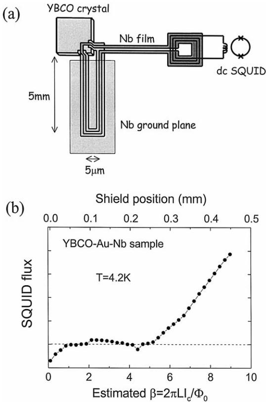
Fig. 6. (a) Variable inductance corner SQUID loop designed to measure the spontaneous flux vs. the inductance parameter  $\beta$ . (b) Preliminary observation of the onset of the SQUID flux as function of the position of the ground plane.
