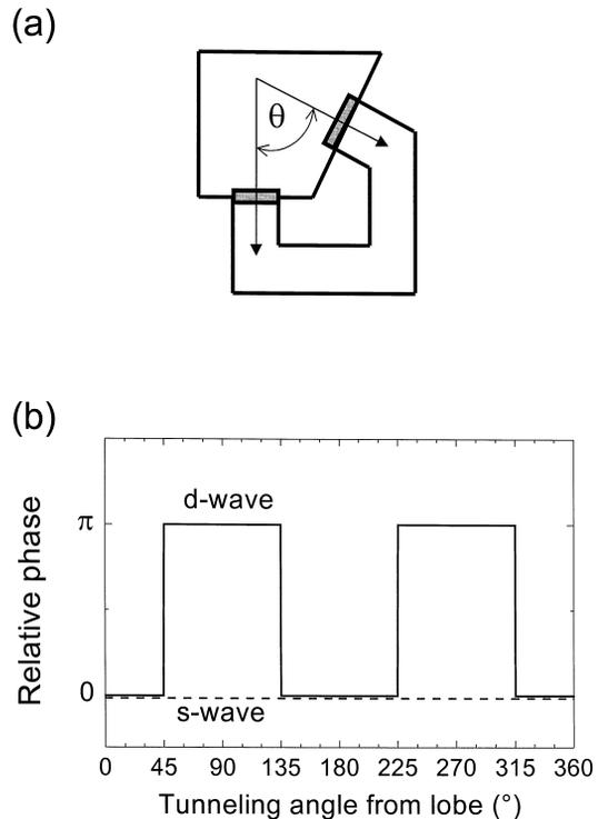
Fig. 3. (a) The SQUID interferometer design for measuring the relative phase of the order parameter in arbitrary *k*-space directions. (b) Expected phase shift as a function of tunneling angle  $\theta$ . For a d-wave superconductor, the phase shift is either 0 or  $\pi$ , switching discontinuously at the nodes.
