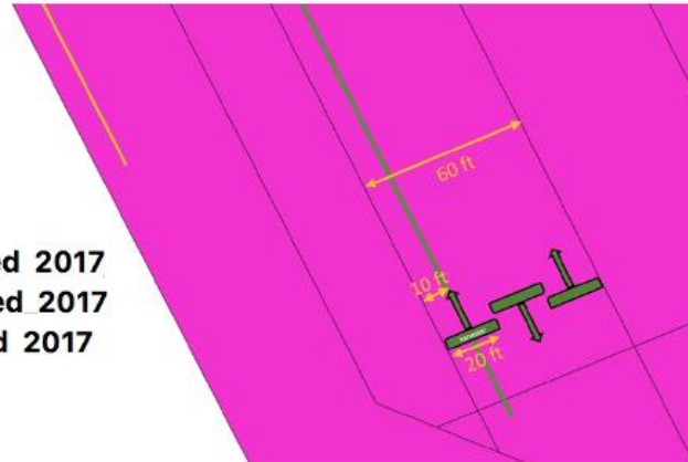
Figure 4. A trial's plot width depends on equipment sizes
