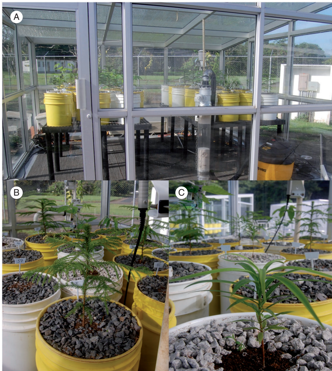
Fig. 1. Glasshouse showing soda lime column and vacuum pump in foreground (A), seedling of Araucaria heterophylla (B) and (C) seedling of Podocarpus guatemalensis .
