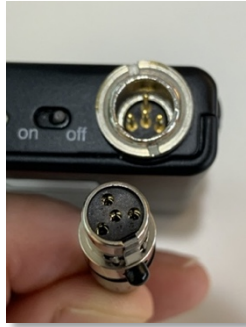
Figure 9 Mic cable and transmitter jack showing pins to be lined up
